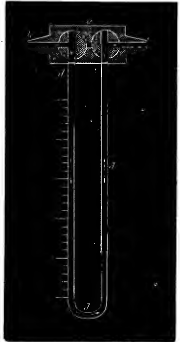
VOLKMANN'S APPARATUS for measuring the rapidity of the arterial circulation.
